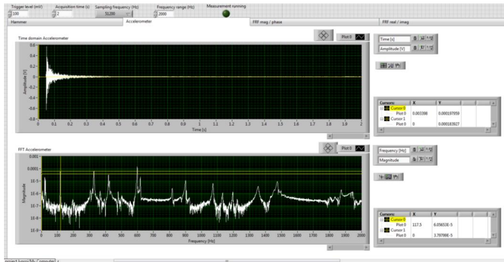
Figure 7 : Time and frequency response expected from the accelerometer on the structure.
